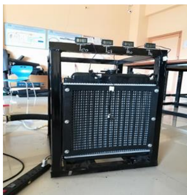
Fig. 2 Radiator with cooling fan
