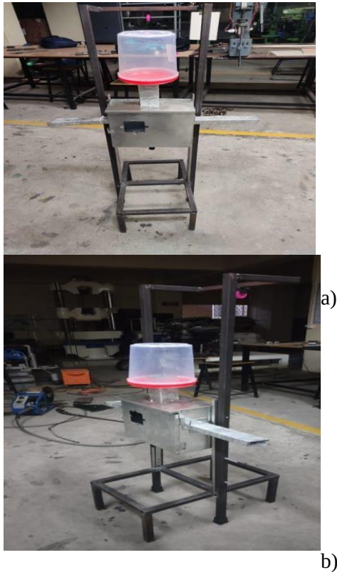
Fig. 7. a) and b) Height adjustment of the scarecrow robot
