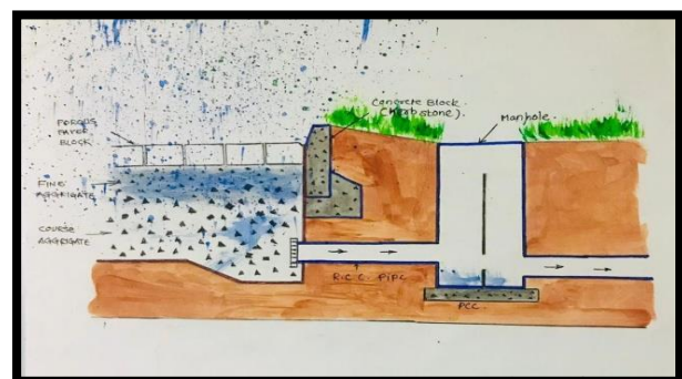
Fig. No. 2 Drainage System For Porous Block
