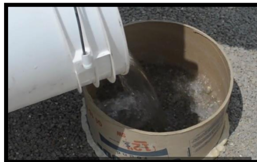
Fig. No. 3 Infiltration Process
