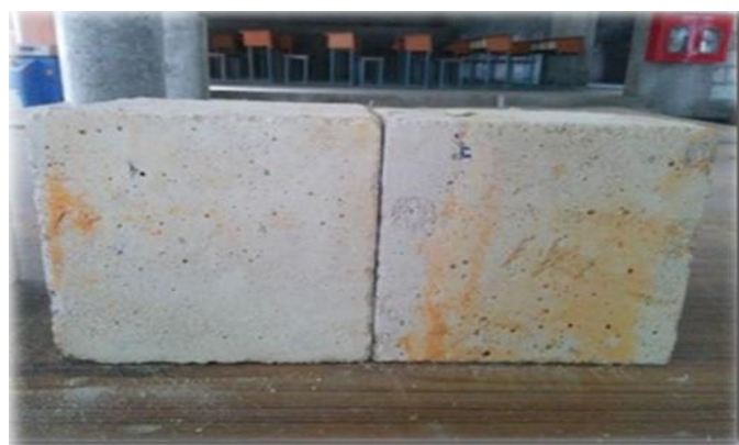
Fig 1: Hydrochloric Acid Attack on Concrete
