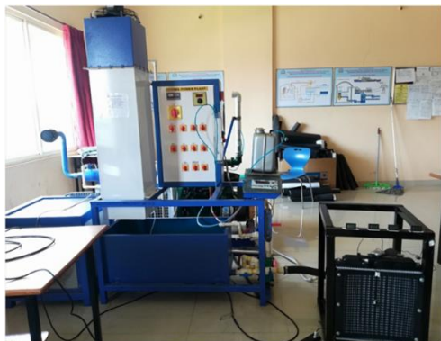
Fig. 1 Diesel Power Plant (Working test rig)
