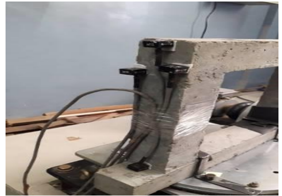
Fig no – 4.0(A) showing arrangement of model on shake table
