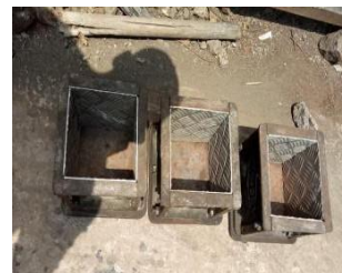
Fig No. 7 (Embossed Plates Mould & Casted Blocks)
