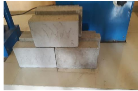
Fig 3. Locking of bricks with one another
