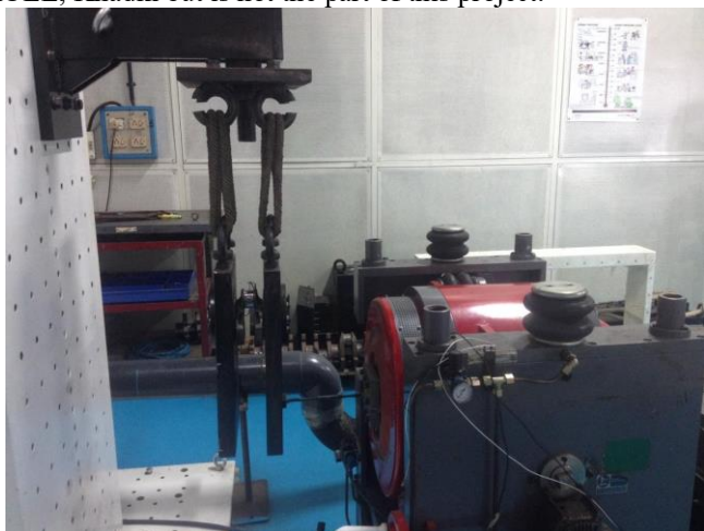
FIGURE . Setup for bending testing.
