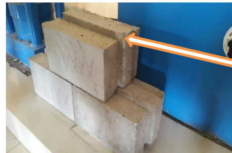
Fig 4. Locking of bricks with one another
