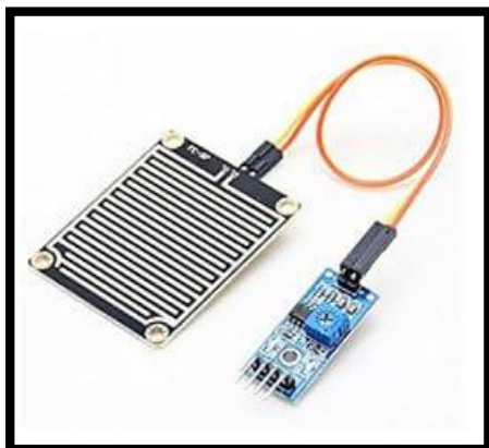
FIGURE – 6. Rain drop sensor module for Arduino
