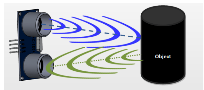
Figure 2: Working of ultrasonic sensor
