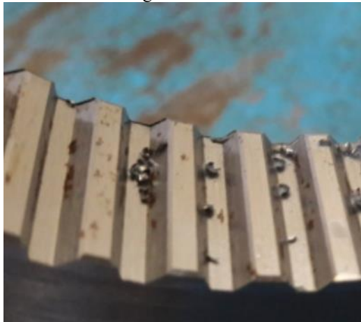
Figure b. Burr on Internal gear
