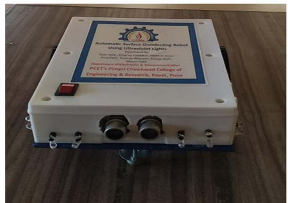
Automatic Surface Disinfecting robot using Ultra Violet Light
