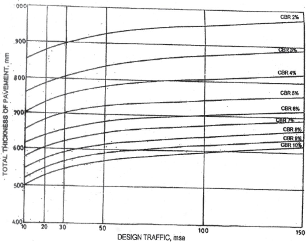
Fig. 2. Pavement Thickness Design Chart for Traffic 10-150 msa
