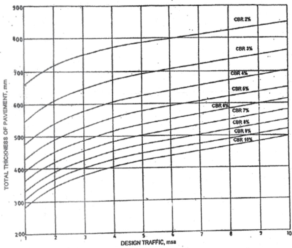
Fig. 1. Pavement Thickness Design Chart for Traffic 1-10 msa
